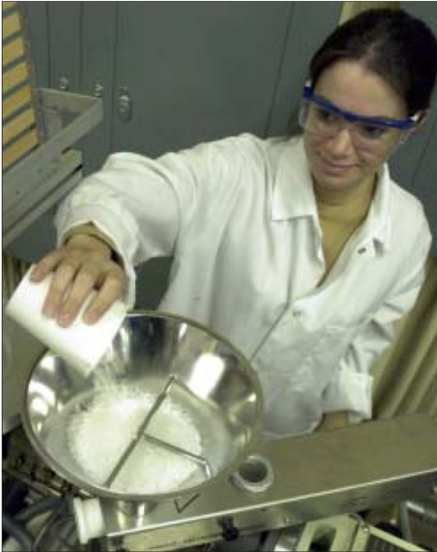
Danielle Froio, a plastics engineer with the Materials Science Team, pours polymer pellets into the ThermoHaake Twin Screw Extruder during a production run of experimental blown-film nanocomposites.
