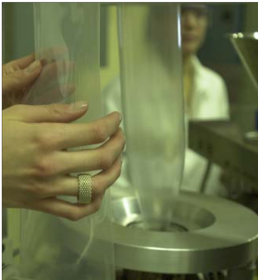
A blown-film nanocomposite flows out of the ThermoHaake Twin Screw Extruder.
